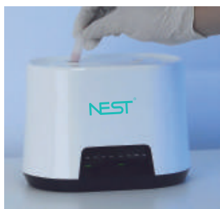
02 Insert the cryogenic tube into the hole
